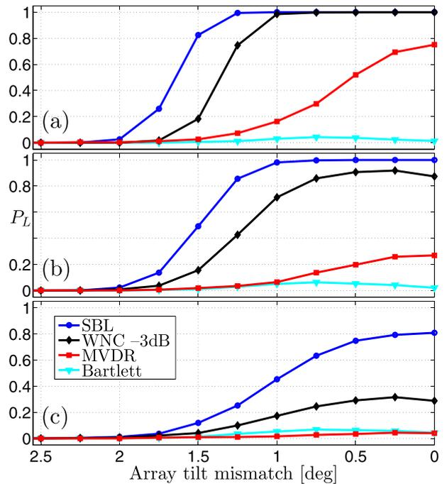
FIG. 5. (Color online) Probability of localizing ( $P_L$ ) the weaker source using multi-frequency (166 and 201 Hz) in the presence of array-tilt mismatch at SNR (a) 0 dB, (b)  $-5$  dB, and (c)  $-10$  dB. Data snapshots are drawn randomly from a finer replica vector mesh for stationary sources.
