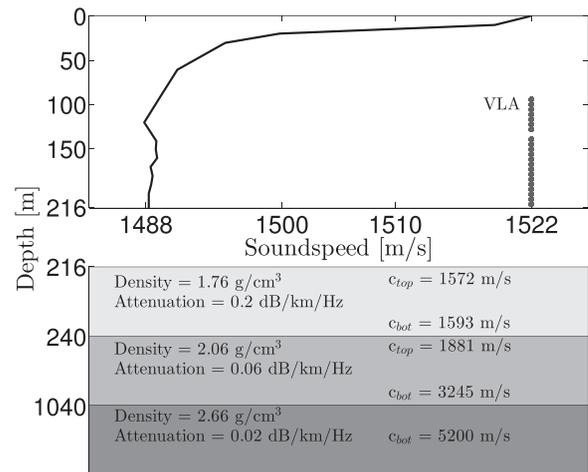
FIG. 2. Waveguide with sound speed profile, VLA, and geo-acoustic parameters for range-independent SWellEx-96 Event S5. A single element out of the 22 element subset is excluded from processing.
