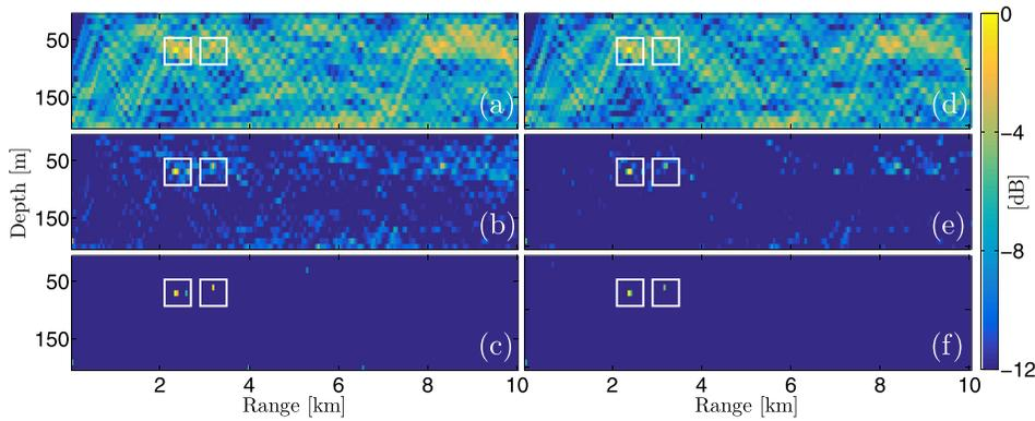
FIG. 8. (Color online) As in Fig. 7 but using two frequencies (166 and 201 Hz) reduces the ambiguous peaks competitive in power to source 1 and source 2 to approximately 5 or less for WNC  $-3$  dB and SBL.
