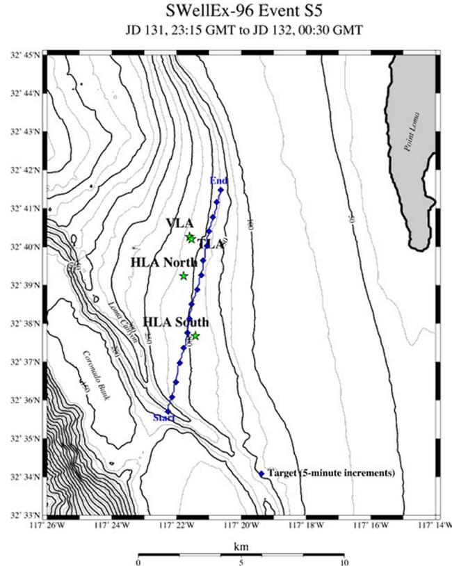
FIG. 1. (Color online) SWellEx-96 Event S5 showing the path of the surface ship R/V Sproul in blue. The ship towed a deep source at  $\sim 60$  m depth along roughly a 200 m isobath during the 75 min VLA recording.
