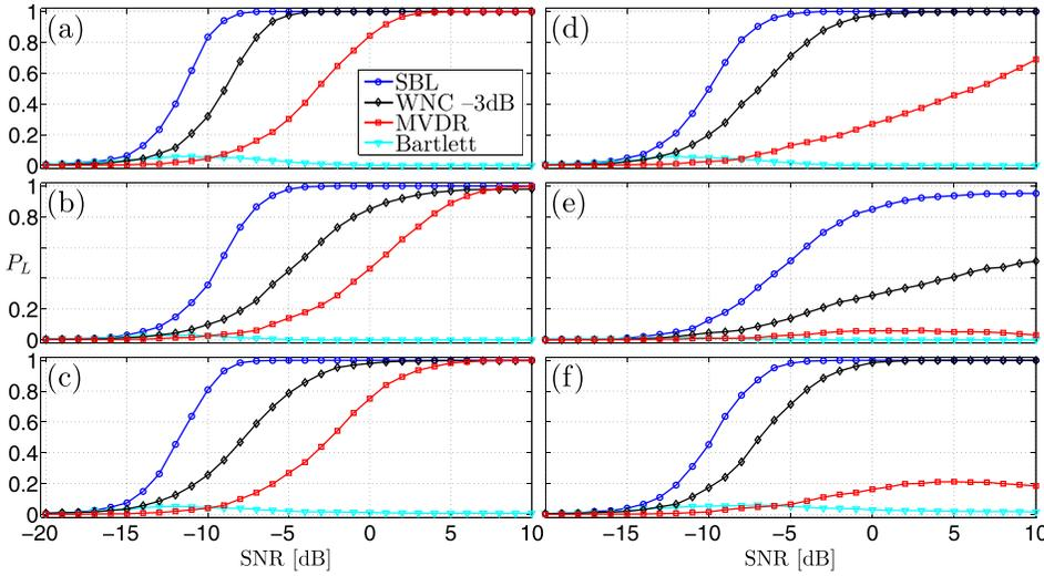
FIG. 4. (Color online) Probability of localizing ( $P_L$ ) the weaker source 2 for 166 Hz [(a), (b), (d), (e)] and two-frequency (166 and 201 Hz) [(c), (f)].  $L = 21$  data snapshots are drawn randomly from a finer replica vector mesh for stationary sources in (b), (c), (e), (f). Left panels are without array-tilt mismatch, right panels include a  $1^\circ$  array-tilt mismatch.
