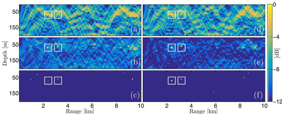
FIG. 7. (Color online) Localization for two SWellEx-96 sources at 166 Hz for data segment 85 of 142. True positions are indicated by white squares. Replica vectors are computed with  $0^\circ$  (left panels) and  $1^\circ$  (right panels) tilt: (a), (d) Bartlett; (b), (e) WNC  $-3$  dB, and (c), (f) SBL. Bartlett displays the most ambiguity while all other processors exhibit fewer ambiguous localizations.
