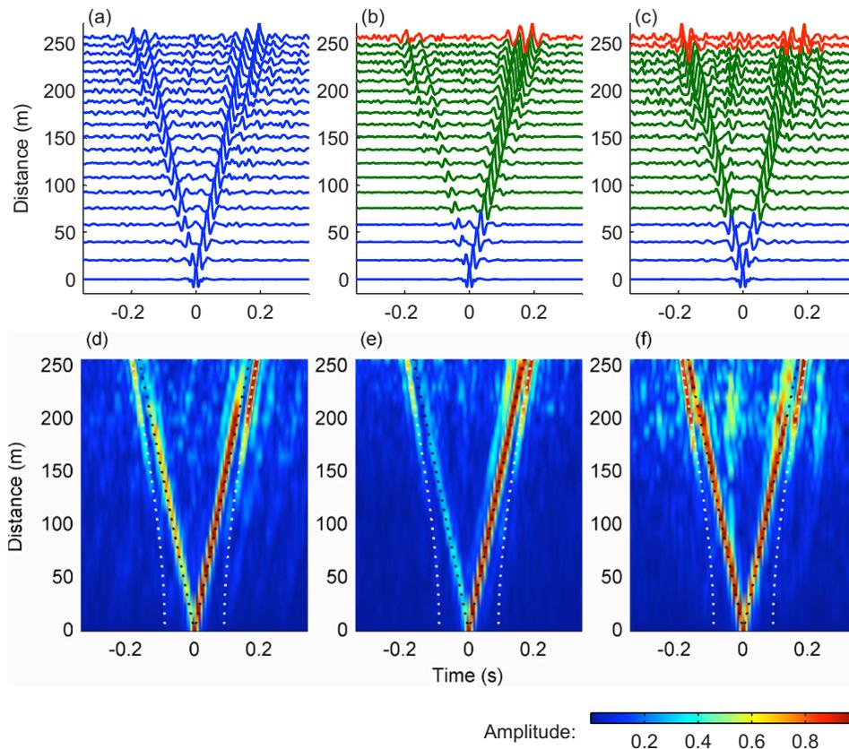
Fig. 4. (Color online) (a)–(c) Cross-correlations between channel 13 (first HLA hydrophone) and all other channels after re-sorting the channels, plotted as a function of distance from hydrophone 13 [(a) before, (b) between, and (c) after switches]. (d)–(f) Normalized envelopes of the cross-correlation function time derivatives, with simulated direct (black dotted lines) and surface reflected path travel times (white dotted lines) [(d) before, (e) between, and (f) after switches].
