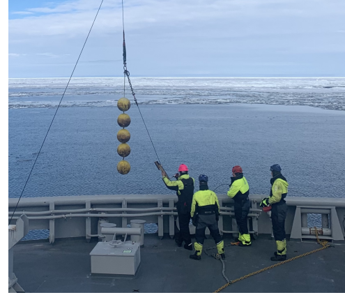
Figure 3.7. Oceanographic mooring CNRS23, shown here being recovered by KV Svalbard , was localized using active acoustics before being released from its anchor. (Photo: Sofia Vakhutinsky)
