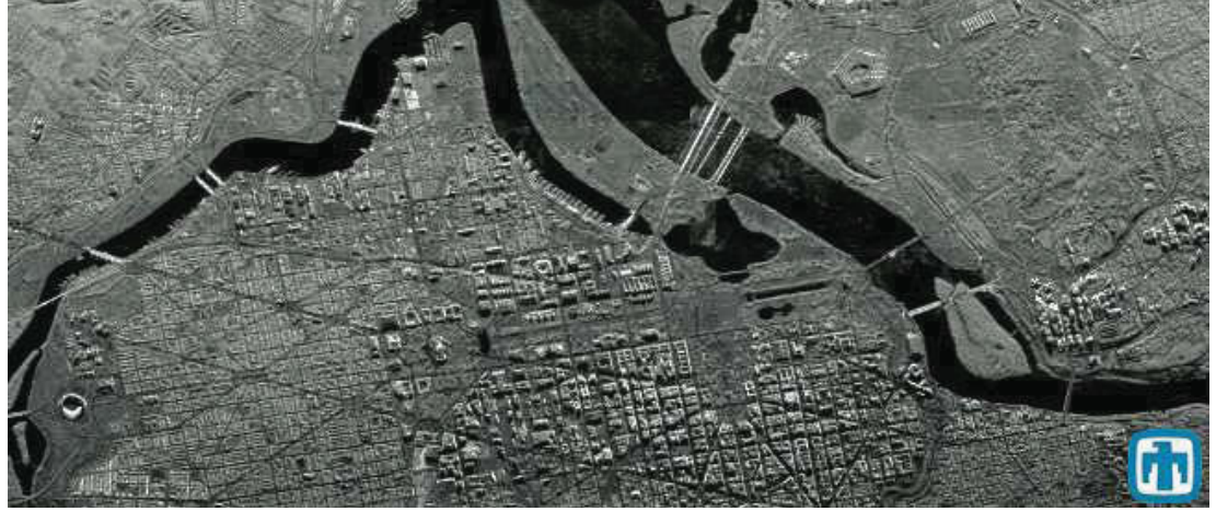
Figure 4.7: 1-m resolution SAR image of Washington, D.C. (Image courtesy of Sandia National Labs, http://www.sandia.gov/radar/imageryku.html .)
