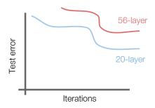
56-layer model performs worse on both training and test error
