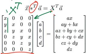
When stride=1, convolution transpose is just a regular convolution (with different padding rules)
