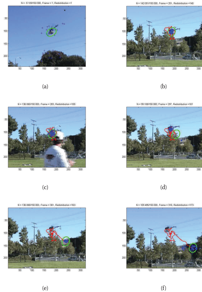
Figure 23.6 Example of particle filtering applied to visual object tracking, based on color histograms. (a-c) succesful tracking: green ellipse is on top of the helicopter. (d-f): tracker gets distracted by gray clutter in the background. See text for details. Figure generated by pfColorTrackerDemo , written by Sebastien Paris.
